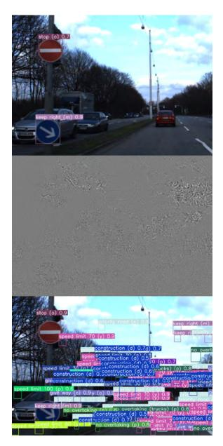
**Figure 9.** Visualization of the overflow on a TSR model. (Top) Normal output of the TSR system: the two signs are detected as expected. (Middle) Amplified intensity of the perturbation added to each pixel of the image. (Bottom) Output of the TSR system on the adversarial image: more than 100 signs are detected with high confidence.
