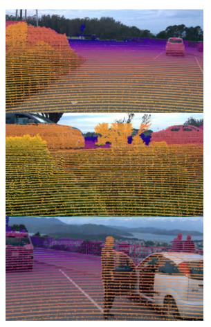
**Figure 5.** Superposition of outputs from cameras (RGB images) and from LIDARs (range maps) (adapted from the Waymo Open Dataset [64]). For the range, the colour is coded from yellow (close) to purple (far).
