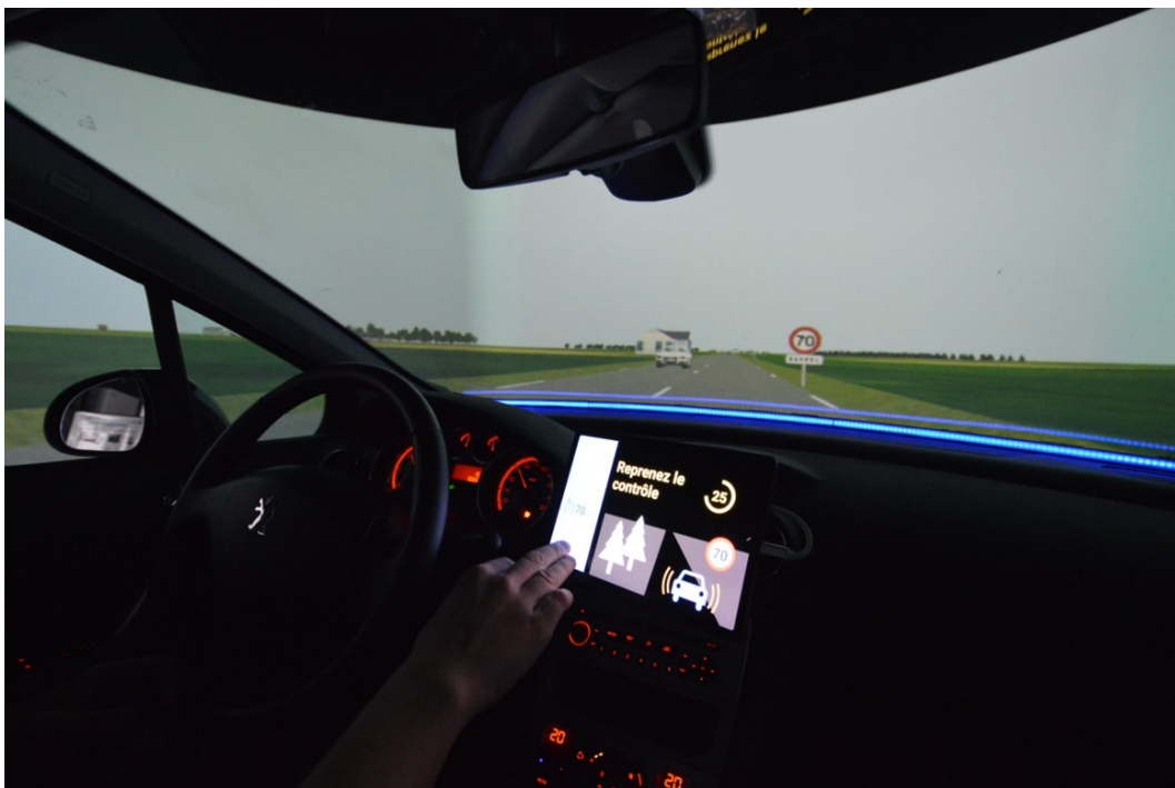
Figure 3.4: UTBM's driving simulator: embedded multichannel HMI
